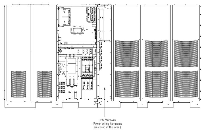
Figure 4-6. ISBM and UPM Sections Joined
